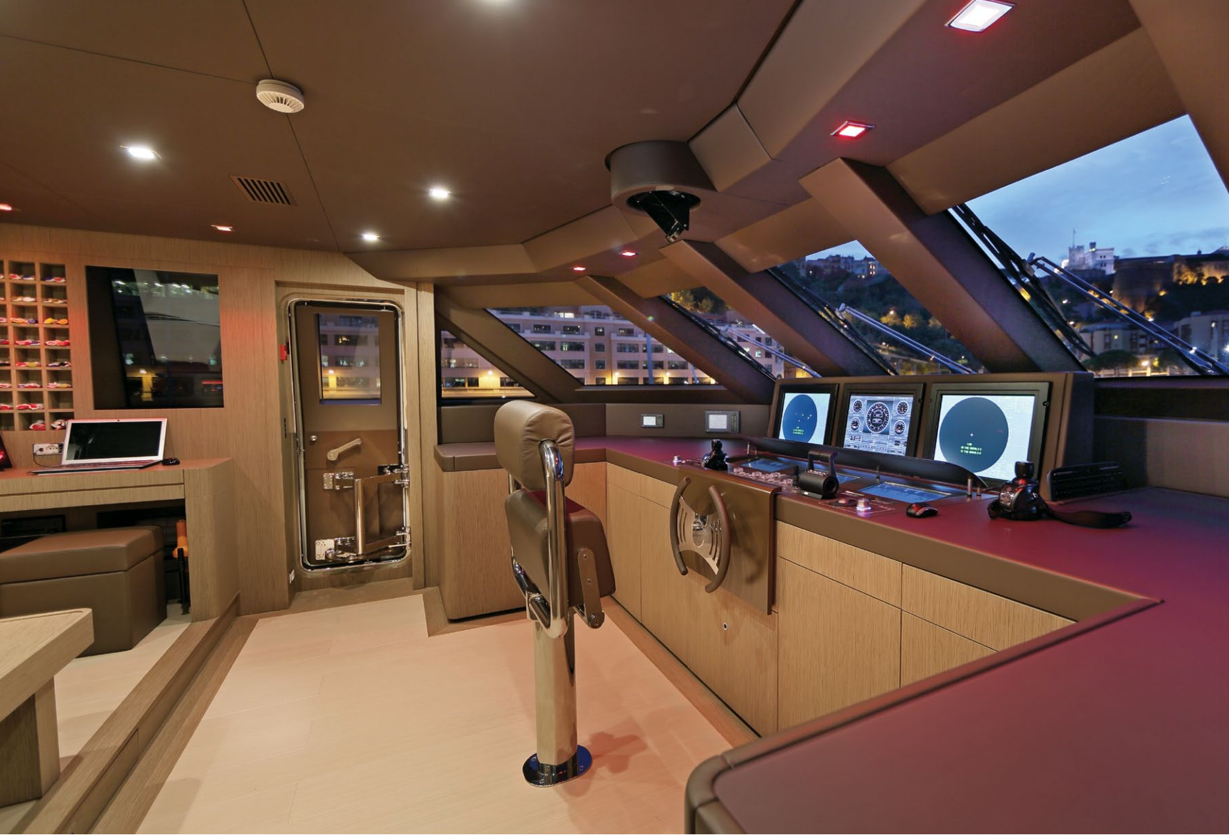
ABOVE: The integrated I-Bridge system by Team Italia provides a clutter-free wheelhouse. In the absence of wing stations, a wireless maneuvering device can be used to pilot the yacht.
